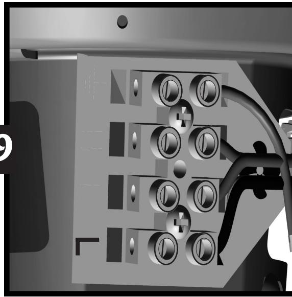
An additional "L" terminal is provided for separate control of the light kit if a separate line is provided for that purpose.
